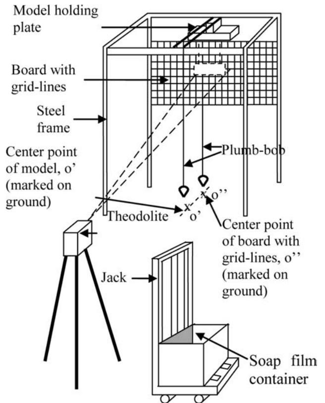
Figure 5: Set-up for the soap film model experiment
