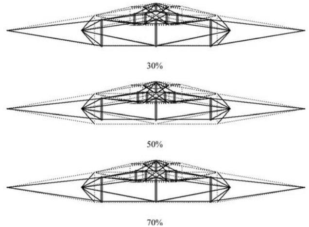
Figure 6: Shape optimal design of the flower e dome with pre-tension
