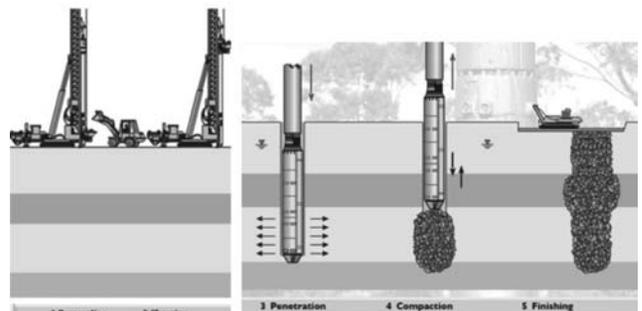
Fig. 2: Process of Vibro Replacement.
