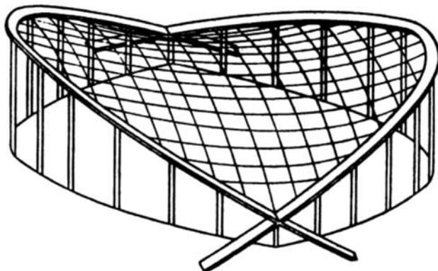
Fig.3 Raleigh Arena cable diagram. Severud Assoc. Struct. Eng.
