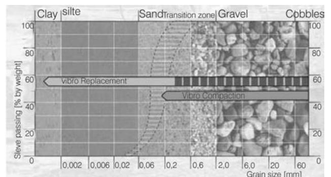
Fig. 1: Particle size distribution illustrating applicability of Vibro Compaction and Vibro-Replacement.
