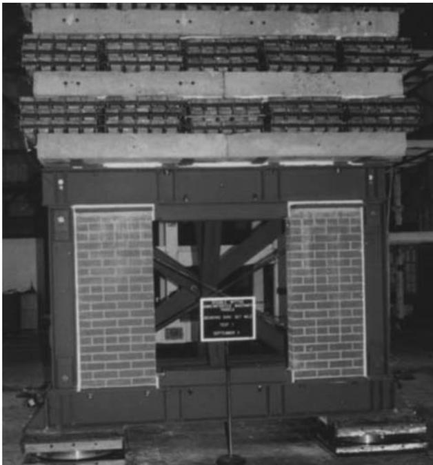
1992 URM Tests: Isolated structure remains undamaged after 58 earthquakes including magnitude 8 earthquake loadings.
