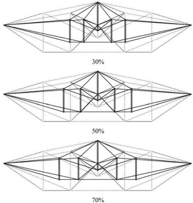
Figure 3: Shape optimal design of the seven-struts cable dome with pre-tension
