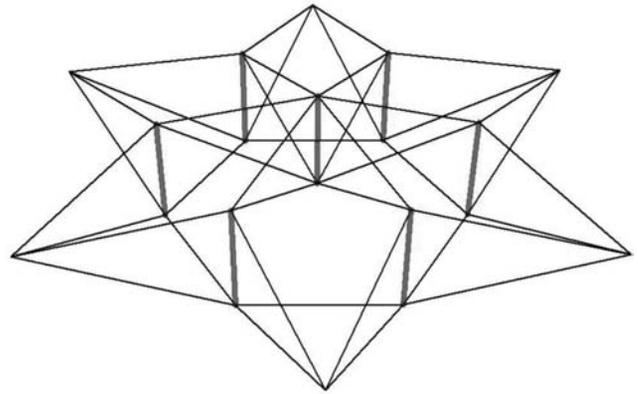
Figure 2: seven-struts cable dome
