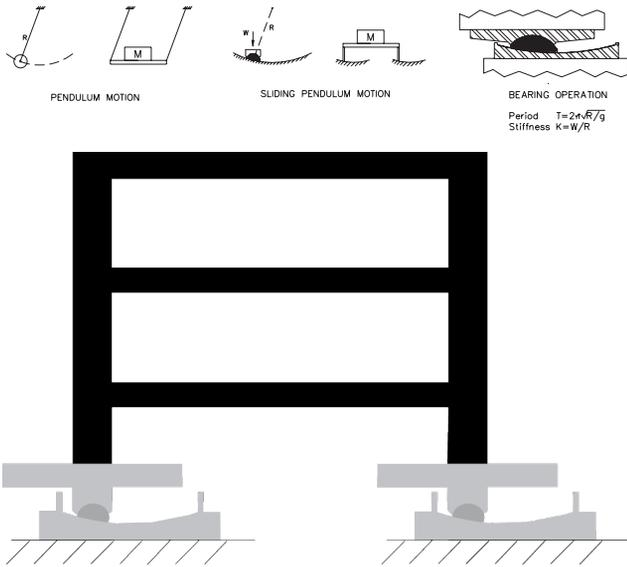
Principles of Friction Pendulum Bearing Operation
