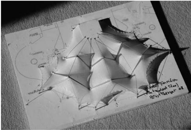
Fig.6 Stretch Fabric Model for Extended Roof 2008
