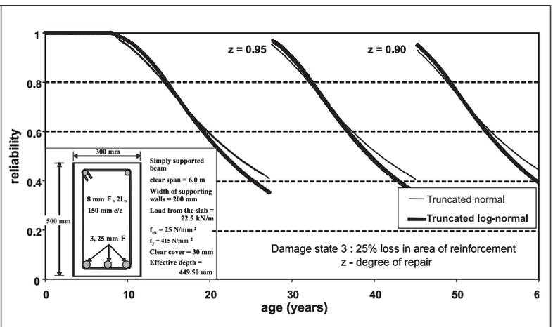
Fig. 8 Reliabilities for the beam against damage state 3
