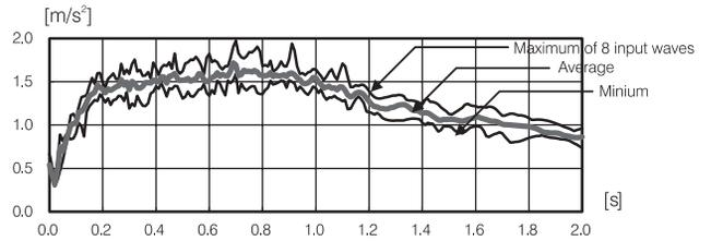
Figure 2: Acceleration spectra of adopted input waves
