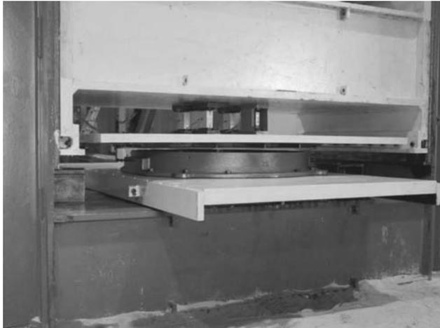
Bearing in Test Machine
