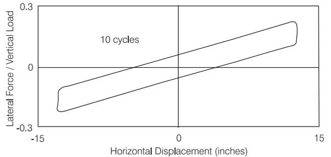
Test Results for 3 and 10 Cycles, respectively, at 1.2x Design Displacement
