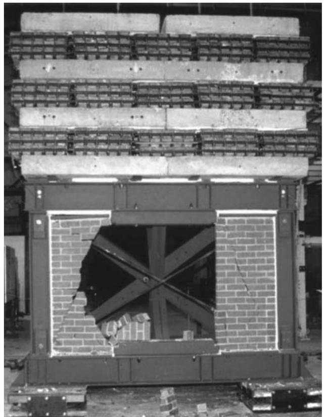
1992 URM Tests: Non-Isolated structure fails after 3 earthquakes of magnitudes 5, 6 and 7, respectively.
