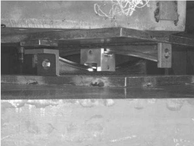
Tension Bearing in Test Machine
