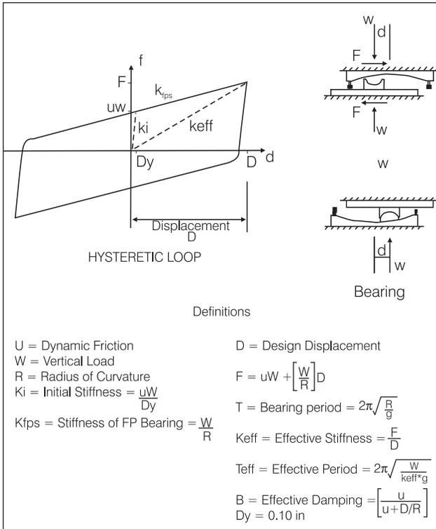
The semi-spherical design of the articulated slider achieves relatively uniform pressures under the articulated slider. The relatively uniform pressure distribution reduces slip-stick motion and prevents high local bearing pressure from occurring. The lateral restoring stiffness of the Friction Pendulum™ bearing is,  $k = W/R$
