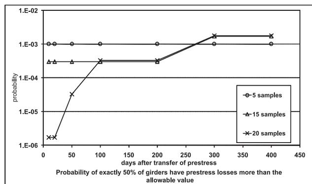
Fig. 5 Probability of exactly 50% of the girders in the bridge stock having prestress losses more than expected prestresses losses (estimated at the design stage using B3 model)
