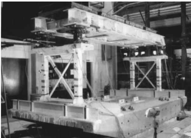
1992 Shake Table Tests of Bridge on Flexible Piers
