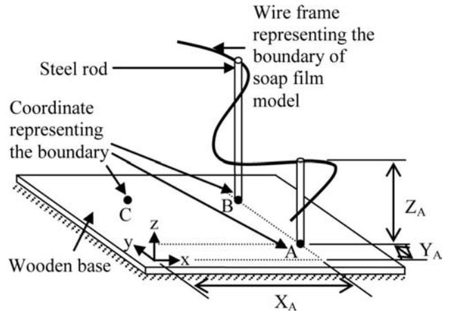
Figure 4: Making of boundary wire frame
