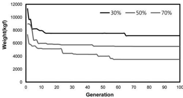
Figure 4: History of optimization with respect to the seven struts cable dome
