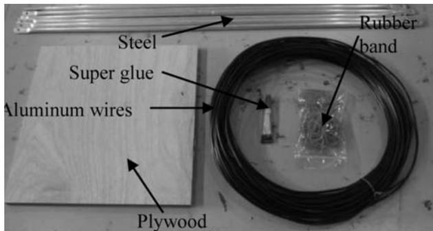
Figure 3: Materials used to build the physical model
