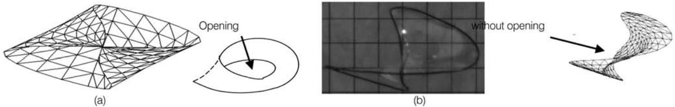
Figure 13: (a) Mathematically defined surface of Möbius strip ( $R/W=1$ ) with opening at the center (b) Soap film model (Möbius strip,  $R/W=1$ )
