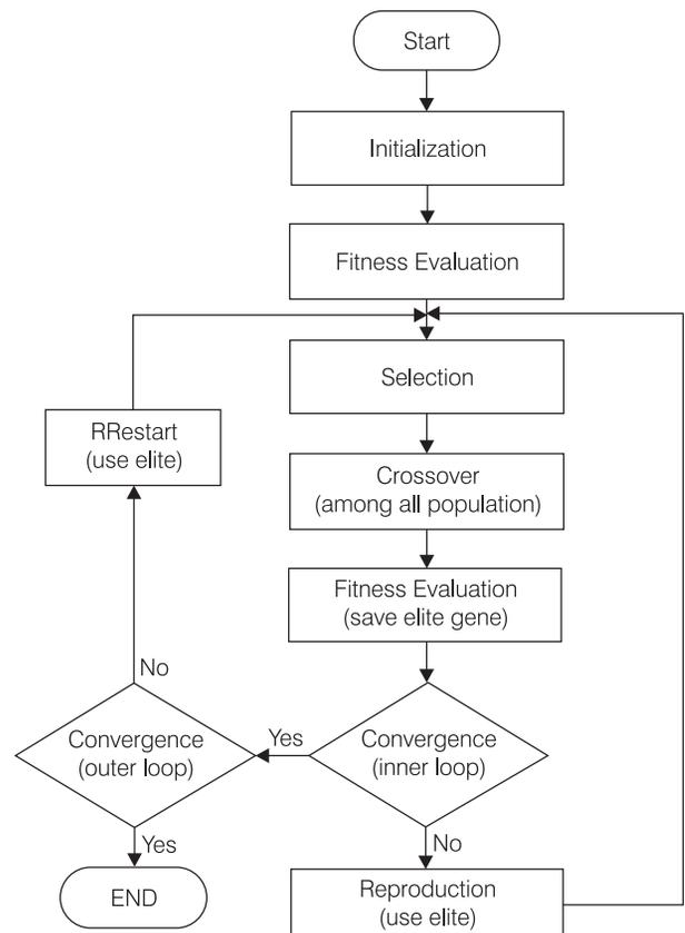
Figure 1: Micro genetic algorithm flow chart
